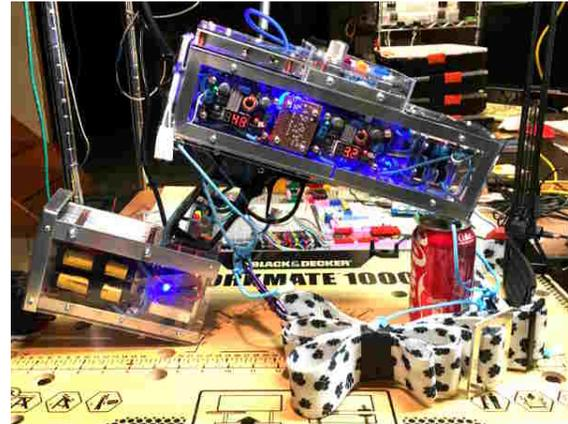
(b) Red LED displays showing 5v and 3.3v are part of two switch mode power supplies.
