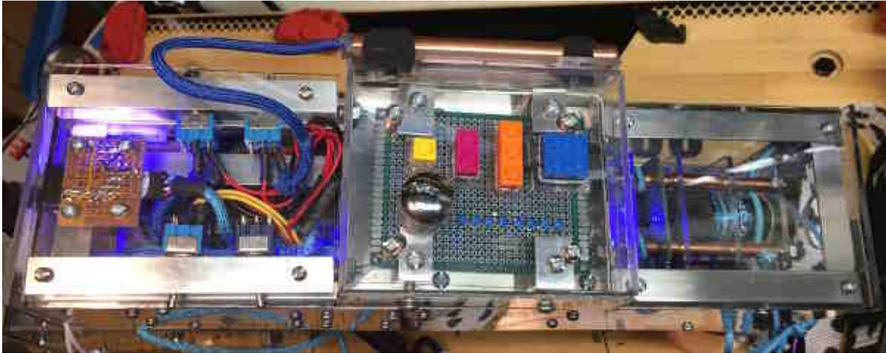
Figure 6. Top view: note Lego® buttons with different sizes for easy touch recognition. Power switches on left, anti-shock bungee elastic mounted LRF on right. Velcro attached copper pencil is an auxiliary alignment laser (Photo by Author)
