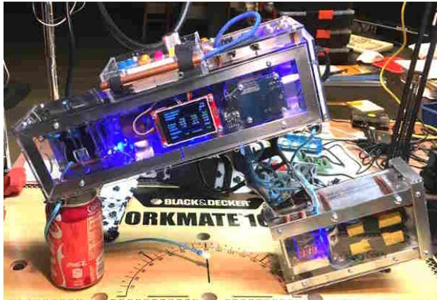
(a) ILI9341 320 x 240 pixel color display. Low voltage alarm/display is below the grip by the yellow batteries.
